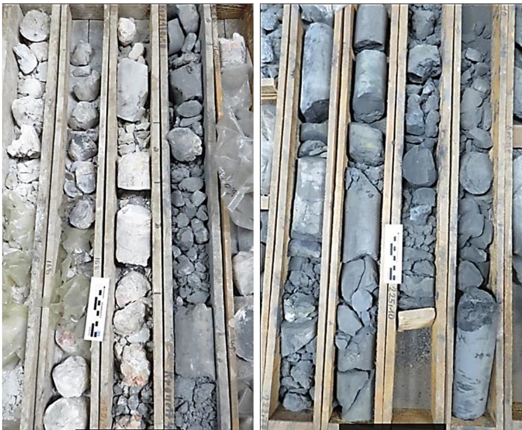
Figure 4-5: Left: 166-177 m, kaolinisation of the core (whitish colour) at the top of dark grey siliceous alteration of basinal Dinantian mudstone. Right: 223-236 m, dark grey siliceous alteration of basinal Dinantian mudstone with white patches of kaolinisation.
